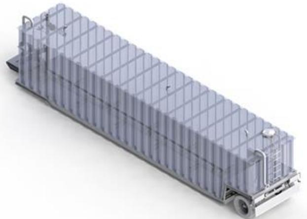
Figure 2: Schematic of a Modular System installed inside an ISO shipping container
