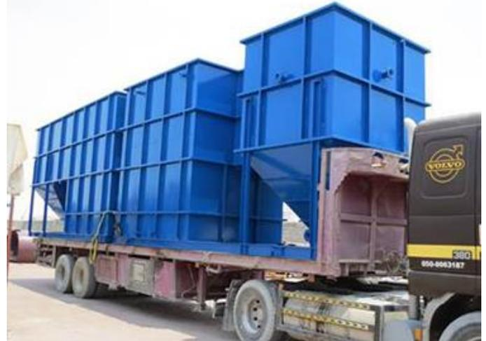
Figure 1: Headworks Modular System transported to site in Qatar
