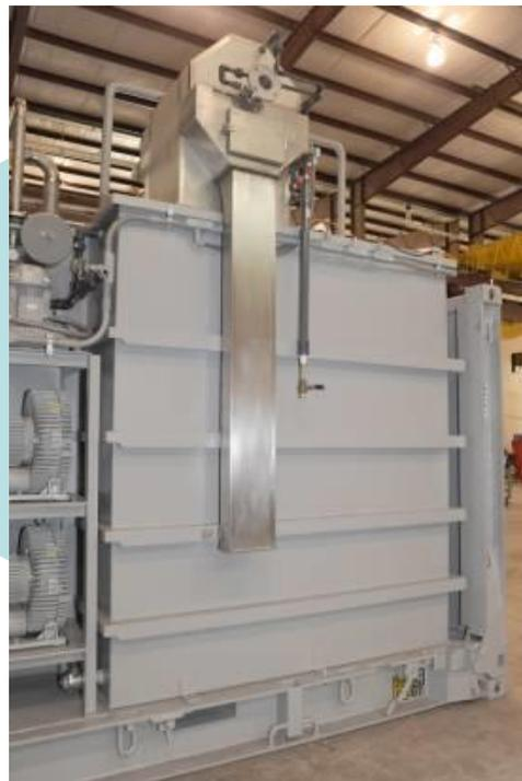
The primary screen is the first stage of the process. It removes coarse solids prior to the influent entering the mixing tank. After mixing, BOD reduction and nitrification occur in the reactors.
