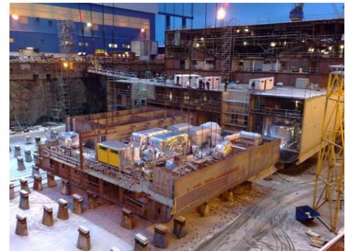
*The CleanSea System installed on the ship's hull during ship building. The biological treatment basins are located in the far corner of the block.*
