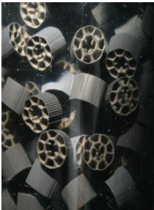
*Biofilms growing on ActiveCell media provide a more resilient, dense treatment population per unit volume compared to conventional suspended growth activated sludge systems.*
