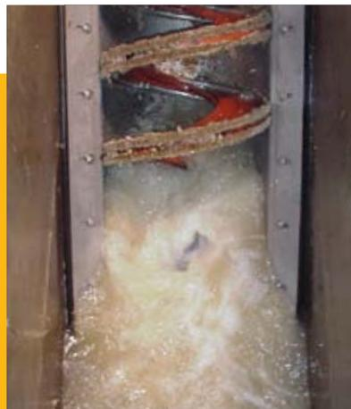
The turbulent zone of influence created by the optional patented TurboWash™ agitator loosens and emulsifies the organic BOD material on screenings.
