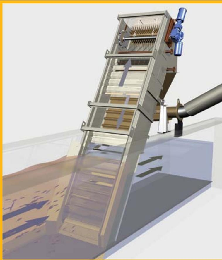
Perforator Screen incorporates sieve elements integrally mounted on a self-lubricating roller chain drive to form a continuous screening belt.
