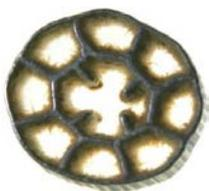
**Figure 2: MBBR Media with Biofilm Attached on the Interior Surfaces**
