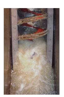
equipment which can include a spiral screen or any other type of screen. Wastewater enters the agitation zone and is heavily mixed. The turbulent zone of influence created by the TurboWash agitator loosens and emulsifies the organic BOD material attached to the screenings allowing the soluble and fine particulate BOD material to pass through the screen openings. Additionally, the screenings device intermittently runs backward thus pushina retained solids back into the
